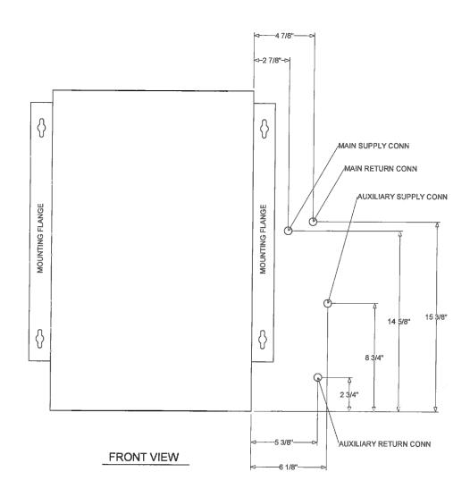
1. PIPING CONNECTIONS ARE 5/8" OUTSIDE DIAMETER COPPER.
